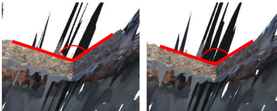
Figure 5.4: Comparison of angles. There should be a difference in angle between un-calibrated, on the left, and calibrated, on the right. Both angles are about 130^\circ though. (They should be 90^\circ .)
