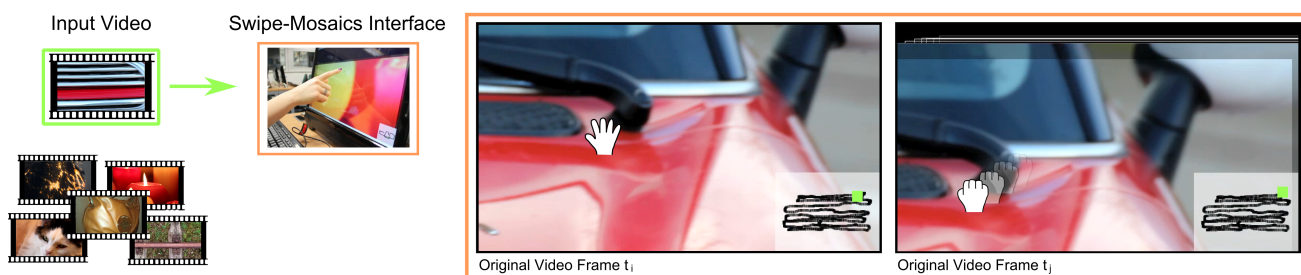
Figure 1: Left : Input videos containing “difficult” phenomena are used as inputs to our system. Right : The Swipe Mosaic interface allowing navigation over an image sequence. We propose Swipe Mosaics as an algorithm and associated interface which composites video frames into a content-centric navigable visualization. Some videos can already be browsed spatially by using existing mosaicing or IBR methods. Our system broadens the range of usable videos because it is trained to tolerate scene motion, parallax, repeated structure, and lack of texture.
