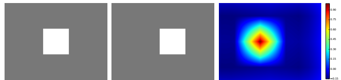
(a) Image pair (left/middle) with strong texture, producing unimodal NCC response (right).
