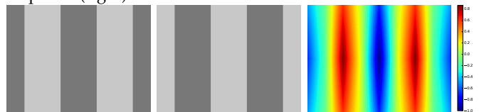
(c) Image pair (left/middle) with repeated structure producing multimodal NCC response (right).
