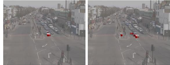
(c) Car detected cutting ahead of traffic.
