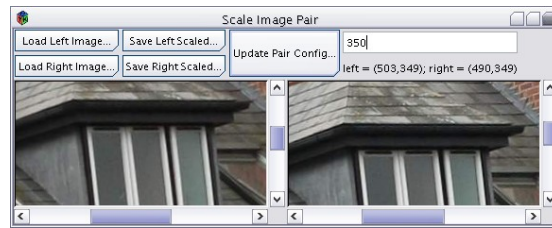
Figure 13: Scaling a rectified image pair.
